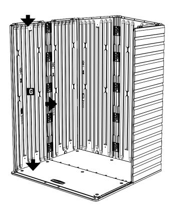
Using a screwdriver, punch out the screw holes on the top of Front Left Side (G) 2 places.
